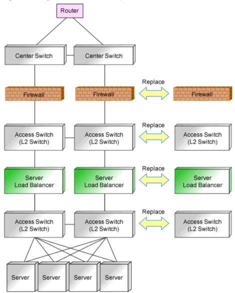
It is premised that you perform replacement while continuing operations using the network devices of redundancy configurations of active and standby switch structure.
